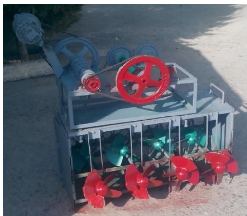
Figure 1. Micro hydroelectric power station based on a water engine.
