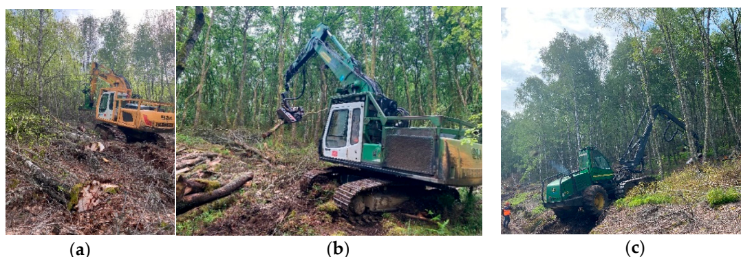
Figure 2. (a) Shear feller-buncher in a medium size Liebherr® 924 RCL tracked backhoe loader; (b) Harvesting head mounted on a medium size Liebherr® R914 LI tracked excavator; (c) John Deere® 1470D wheeled harvester with Waratah® H4415X harvesting head.
