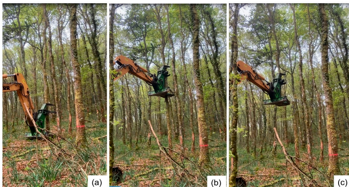
Figure 4. Feller-buncher working with oaks in two stages: (a) head movement for felling; (b) positioning before high cut T_1 ; (c) high cutting T_1 and removing upper stem part. Cutting and the stump height ( T_2 ) is not shown in this sequence.
