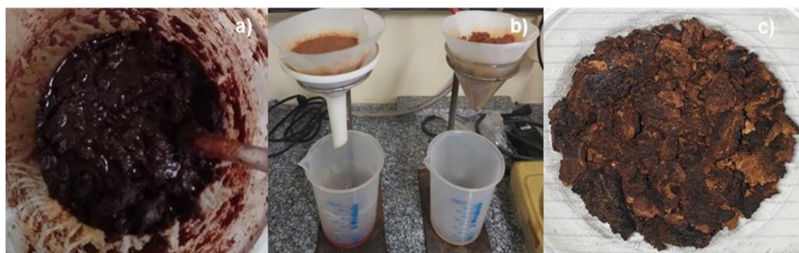
Figure 4. Chemical activation of dried, grinded and sieved Açaí seeds with 2.0 M KOH solution [Açaí seeds fine powders mixed with 0.5 M, 1.0 M, and 2.0 M KOH solution (a); washing/filtration of Açaí pasty cake (b); KOH activated Açaí fine powders seeds (c)].
