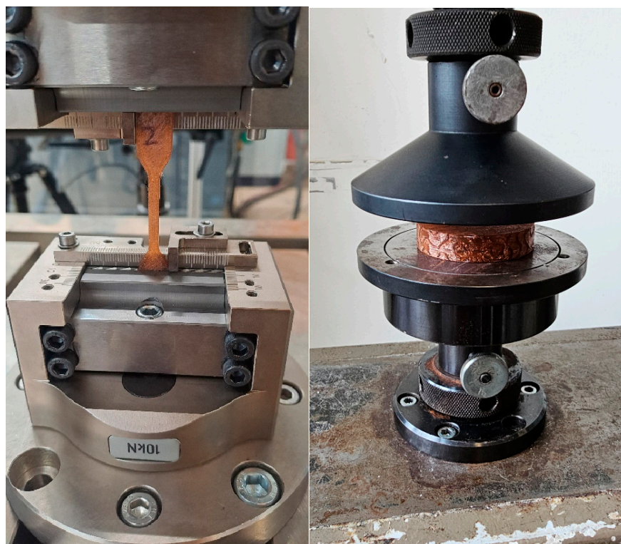
Figure 3. Mechanical Tests on OVERTUE TPU Specimen: left: Tensile test on specimens 5A (DIN ISO EN 527-2); right: compression test.
