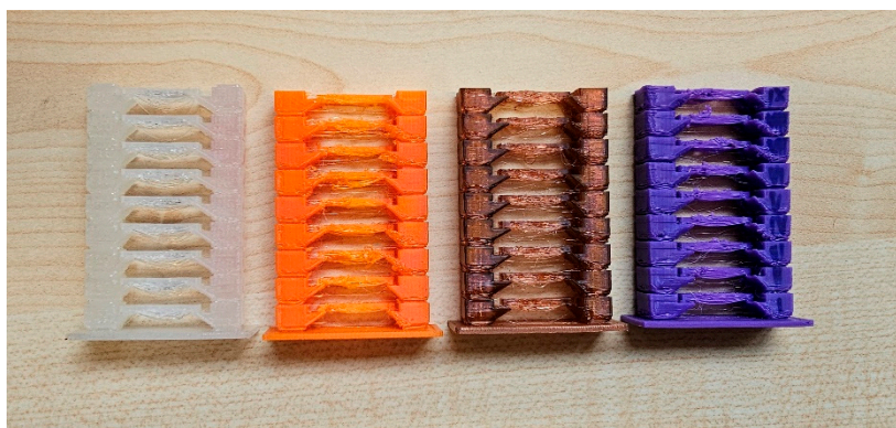
Figure 1. Exemplary illustration of temperature towers made of SemiSoft (transparent), SUNLU (orange), GEEETECH (brown) and OVERTURE (purple) TPU filaments. Temperatures were varied in each step. Printing errors such as stringing are clearly visible at different temperature settings.
