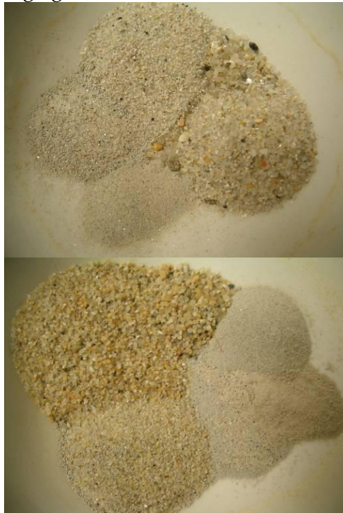
Figure 5. Insoluble fraction of individual mortars obtained after acid dissolution (a) FPo-2, b) FPo-8, c) FPo-10a, d) FPo-10b, e) FPri-A1P1a, f) FPri-A1P1b, g) FPri-PB, h) FN-V2P1.
