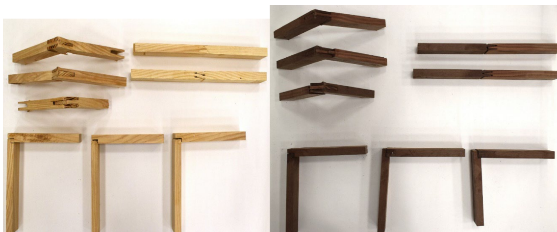
Figure 9. Joints of ash wood: a-native; b-thermal treated.
