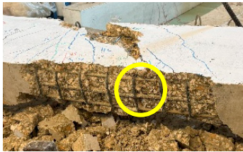
B11-GF-BF (hybrid GFRP-BFRP reinforced beam): GFRP rupture and concrete crushing
