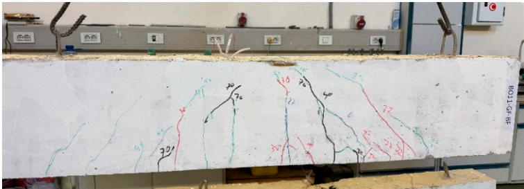
B11-GF-BF (hybrid GFRP-BFRP reinforced beam): GFRP rupture and concrete crushing
