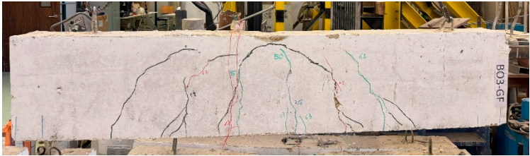
B03-GF (GFRP reinforced beam): GFRP rupture and concrete crushing
