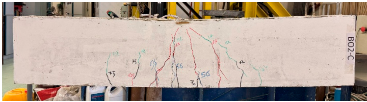
B02-C (control beam): steel yielding and concrete crushing
