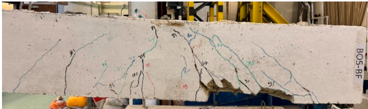
B05-BF (BFRP reinforced beam): BFRP Debonding and concrete crushing
