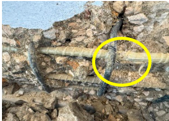
B05-BF (BFRP reinforced beam): BFRP Debonding and concrete crushing
