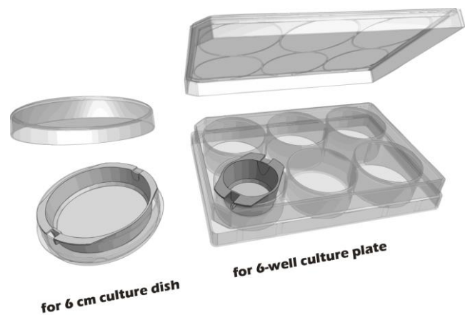
Figure 11. Custom-made culture inserts designed for 6-cm culture dishes and 6-well culture plates.
