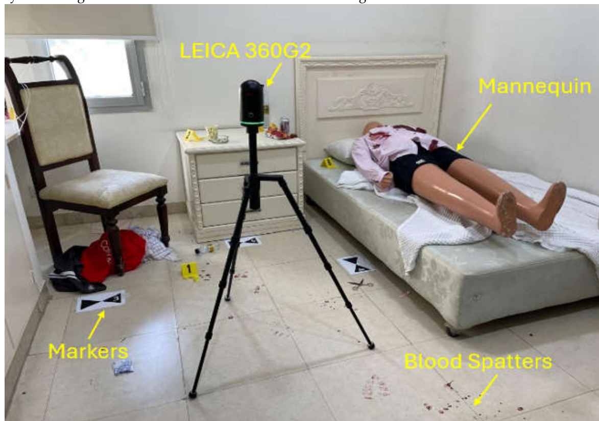
Figure 1. A mock-up crime scene, showing a mannequin, markers, blood spatters, and a LiDAR scanner for ground truth comparison. The scene was prepared by crime scene professionals and has been utilized for training law enforcement officers.
