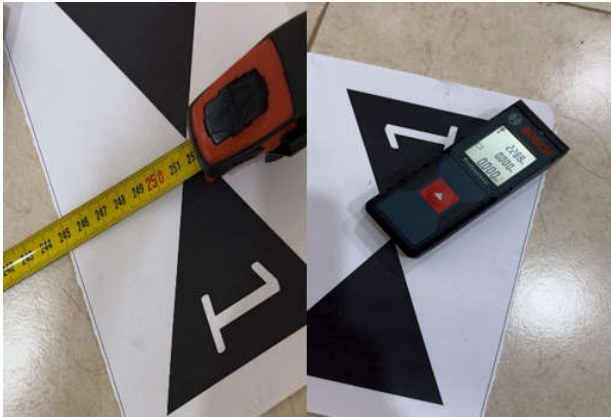
Figure 2. A laser ruler and tape measure are used to measure between markers.
