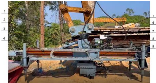
Figure 6. Actual diagram of the device. 1. Heading angle (yaw) rotary device of the aerial platform; 2. Pitch angle (pitch) driving cylinder of the aerial platform; 3. Main beam of the aerial platform; 4. Support leg hydraulic cylinder; 5. Grooving spiral cutter; 6. Spiral cutter rotary device; 7. Spiral cutter sliding pair; 8. Grooving power drive sprocket and chain; 9. Spatial 3D sensor and MCU controller.
