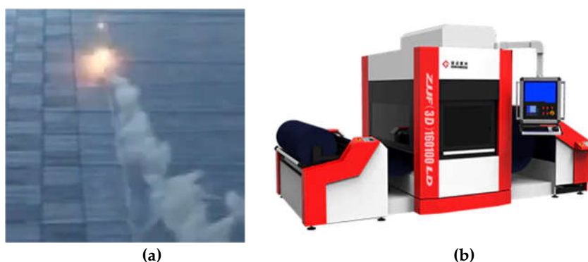
Figure 1. Golden Laser Roll-to-roll System for continuous textile processing; (a) directed CO 2 laser beam; (b) Galvano laser roll-to-roll engraving machine [30,31].
