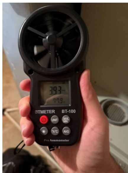
Figure 6. - Intermediate Airflow Test Closer to Ductwork (Test 2).
