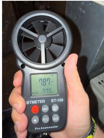
Figure 7. - Increased Airflow Test in Proximity to Ductwork (Test 3).
