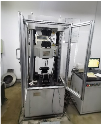
Figure 3. Tensile test of rebar.
