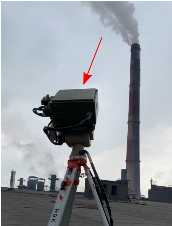
Figure 2. The experimental setup during the measurements. The red arrow shows infrared radiation in the from the chimney exhaust gases.
