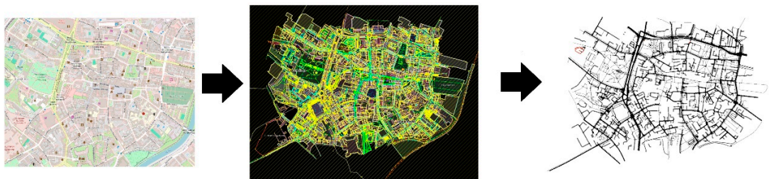
Figure 8. The process of generating data for the map to simulate electric vehicle traffic in SUMO.
