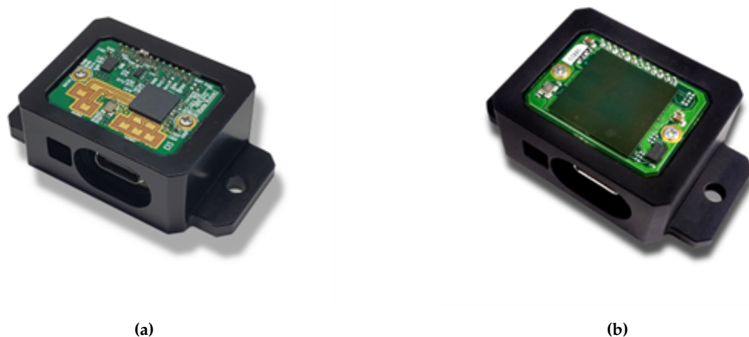
Figure 6. (6a) External Antenna mmWave Base Radar Product [58]. (6b) Antenna on package mmWave Base Radar Product [58].
