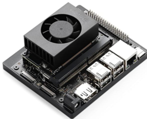
Figure 12. NVIDIA Jetson Orin Starter Kit for platform evaluation.
