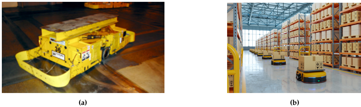
Figure 3. (3a) Legacy AGV for manufacturing applications. (3b) More modern AGV product commonly seen in warehouse automation applications.
