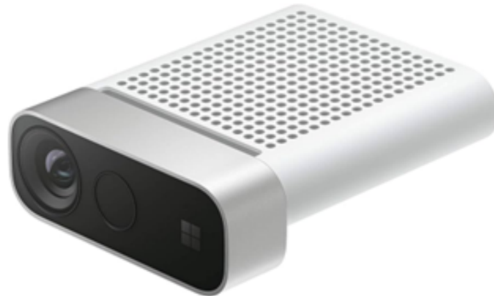
Figure 4. AKDK 1 MP, 120°FOV, 3-D ToF Camera
