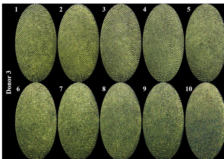
Figure 7. Depletion series developed with the Cu composite from donor 3.
