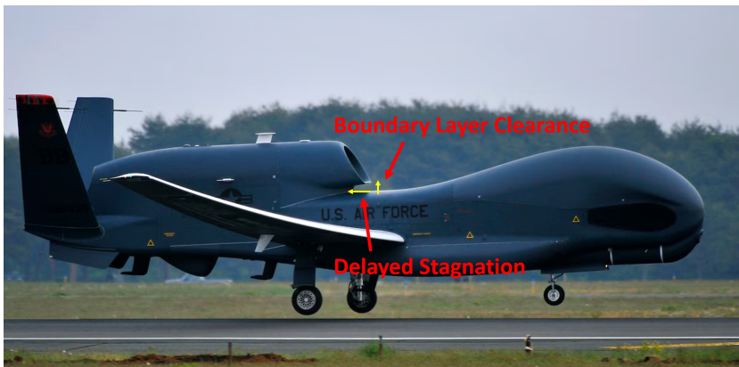
Figure 13. Image of RQ-4 Globalhawk showing engine inlet clearance and overhang for delayed stagnation [46].
