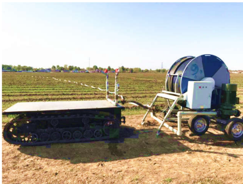
Figure 2. A prototype of the self-propelled hard hose traveler.
