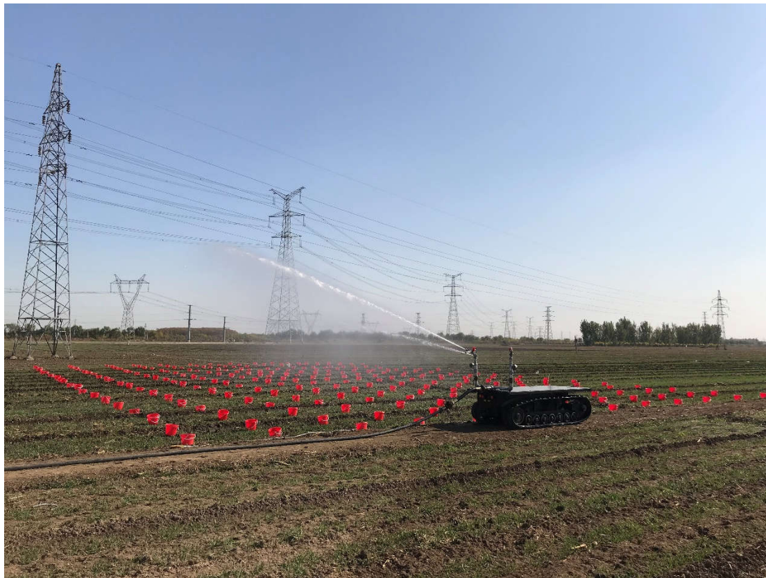
Figure 5. Water buckets and the sprinkler irrigation experiment.
