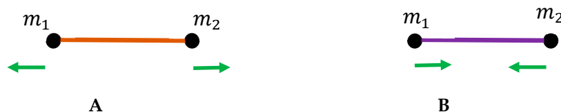
Figure 2. Coloring procedure is illustrated. A. Particles m_1 and m_2 move away or remain at the same distance \frac{d(r_{12}(t))}{dt} \geq 0 is true. Particles are connected with an orange link. B. Particles m_1 and m_2 converge, \frac{d(r_{12}(t))}{dt} < 0 occurs. Particles are connected with a violet link. Green arrows illustrate directions of the particles motion.
