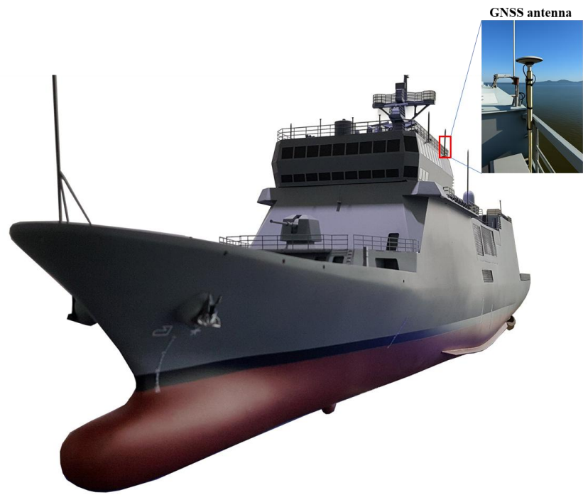
Figure 1. The installation location and physical configuration of the GNSS Antenna on the HANS ( https://bemil.chosun.com/nbrd/bbs/view.html?b_bbs_id=10158&pn=1&num=5439 ).
