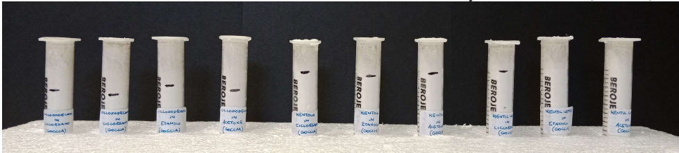
Figure 13. Mock-ups during the test for evaluating the capacity of penetration of VBM.
