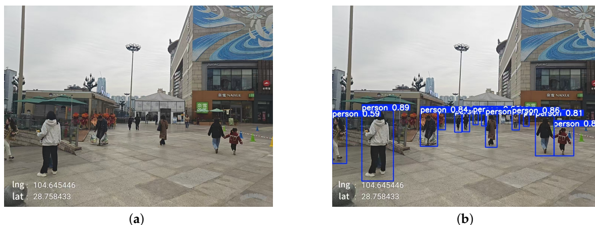
Figure 9. Pedestrian Detection:(a) Original Image;(b) Result Image.
