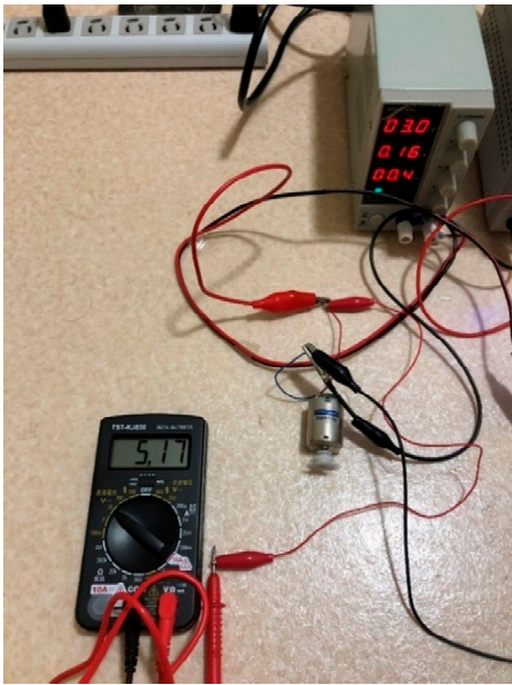
Figure 9-3. A result of the experimental setup in Figure 9-2. When the voltage source displays 3.0 V, the voltage associated with the emergent electric potential is 5.17 V, approximately 40% larger than the source voltage.
