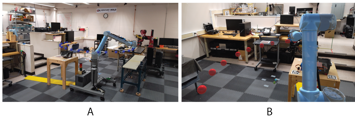
Figure 21. Spheres to show the robot end effector's movement. (A) Blue spheres when the human is in a safe proximity to the robot. (B) Red spheres when the human is in close proximity to the robot.
