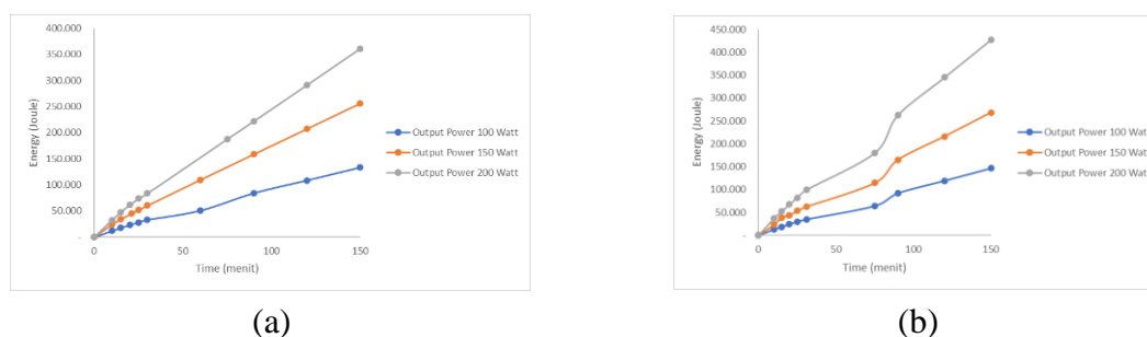
Figure 3. The effect of ultrasonic power on the energy increase polymerization with (a) KOH and (b) NaOH catalysts.
