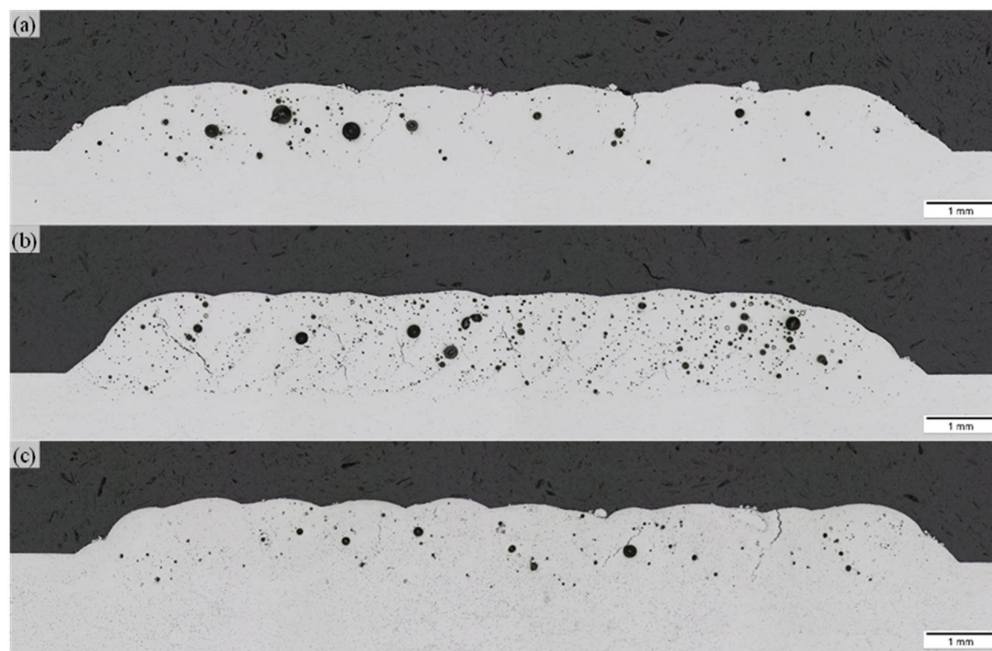
Figure 10. (a) Cross-sections of DED single layer coating (a) hatch = 40%; (b) hatch = 50%; (c) hatch = 60%.
