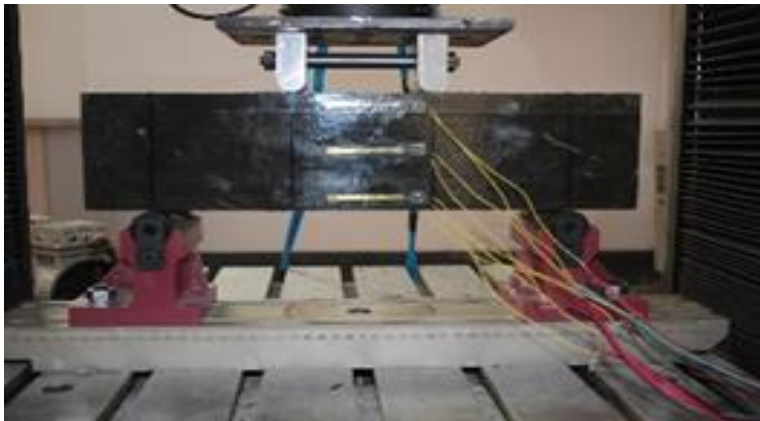
Figure 2. Flexural test diagram of polyurethane concrete material.
