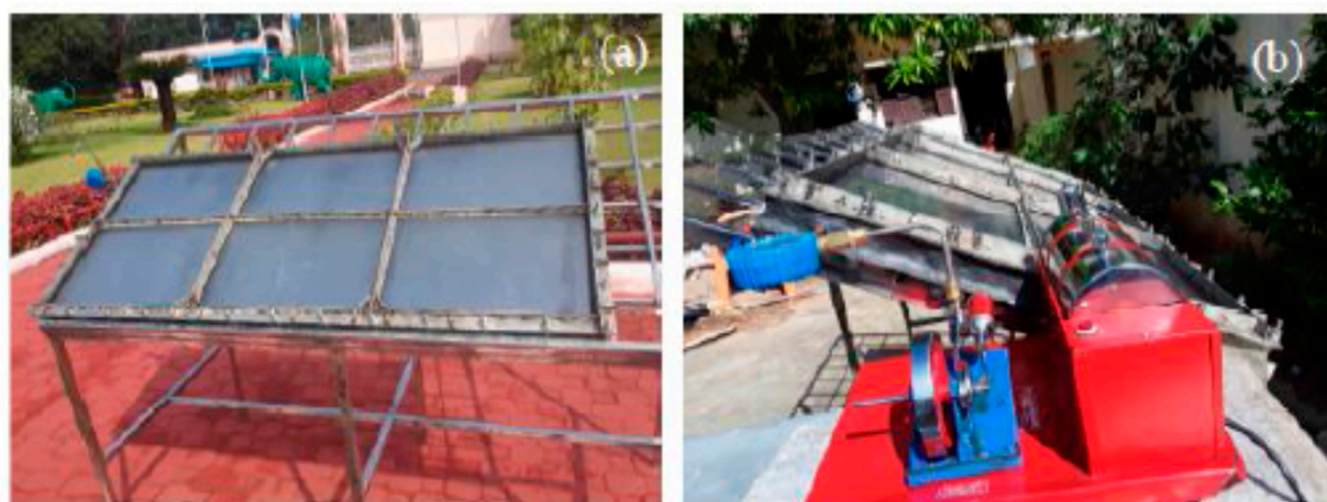
Figure 9. (a) SLAPE solar panel containing about 30 SPV cells with a packing factor of about 100% and about 2 litres \gamma butyrolactone solution and (b) the SLAPE panel connected with reciprocally moved steam engine (RMSE) but not with electric generator [1].
