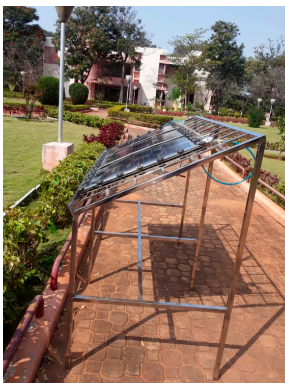
Figure 8. The volume of the SLAPE solar panel 100 before (a) and after (b) exposing to the sunlight for more than 60 minutes when the 0.5 mm thick Al sheet was employed to separate the top and bottom chambers, where the top chamber containing 21 SPVCs immersed in 9.6 litres of \gamma -butyrolactone (NWF 123). The average solar insolation was about 80 mW/cm 2 and the average room temperature was about 28°C [1].
