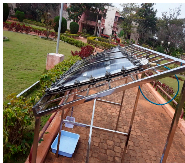
Figure 7. A digital photograph of the sunlight-to-heat energy generating SLAPE solar panel. Panel is placed with an inclination of 30°; (a) front view, and (b) rear view; (c) block diagram showing the generation of electricity from sunlight using a SLAPE solar panel [1,126].
