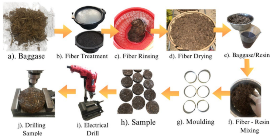
Figure 2. Bagasse Composite and Sample Preparation.
