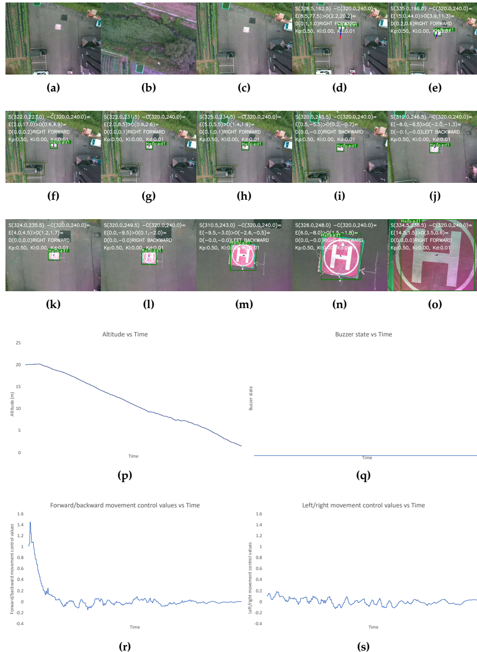
Figure 8. Output for the optimum landing scenario. The images show the (a-o) image frames captured by the camera during different states of flights, graphs for the: (p) altitude, (q) buzzer state, and the control values of (r) left/right and (s) forward/backward movement of the UAV with time throughout landing process. The different state of flight in (a-o) are: (a) after take-off is completed (b) after first way-point is reached (c) after final way-point is reached (d) when autonomous landing is started (e-f) while the UAV is moving to make landing pad appear at center (g-n) after the center of frame and position of landing pad have discrepancy of less than 2m (o) when the UAV altitude is less than 1m and "LAND" command is sent to flight controller
