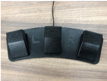
Figure 3. Foot switch of 3-pedal type. Size: 365 mm (W) × 143mm (D) × 41 mm (H), Weight:382g, Switch:Photoelectric switch, Interface:USB, Cable length:2m, Rating:5V/60mA, Service life:>2 million times.
