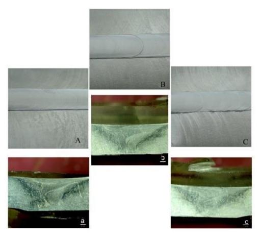
Fig3. Weld surface and the cross-section in different conditions of welding (a) room temp (b) 75 °C (c) 125 °C
