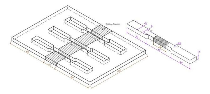
Fig. 2 Schematic view of tensile test specimens prepared from welded plates
