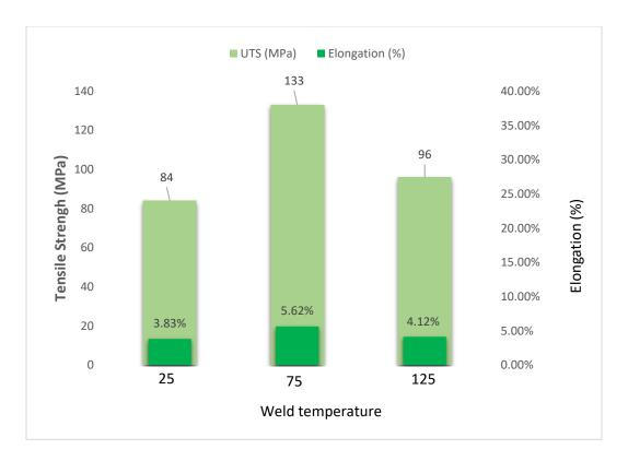
Fig 6. The results from strength and elongation of welded samples.
