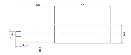
Fig.1 The tool dimensions
