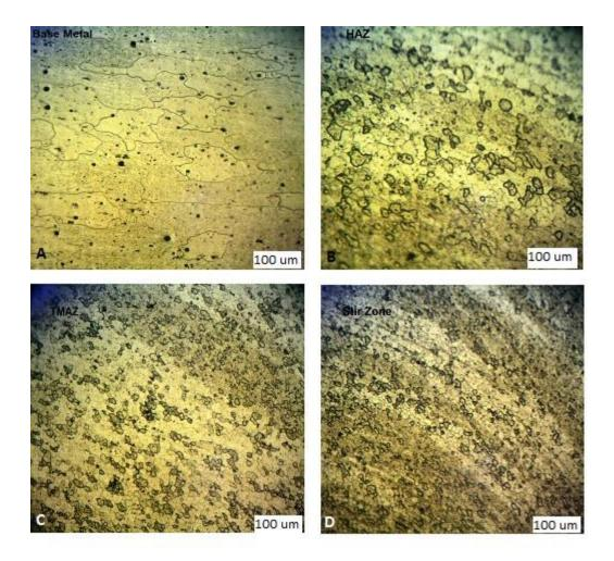
Fig4. Microstructure of aluminum 6061: a. BM, b. HAZ, c. TMAZ and d. SZ (welding condition of  $\omega$  =1200  $\nu$  =75 & preheated in 75 °C)
