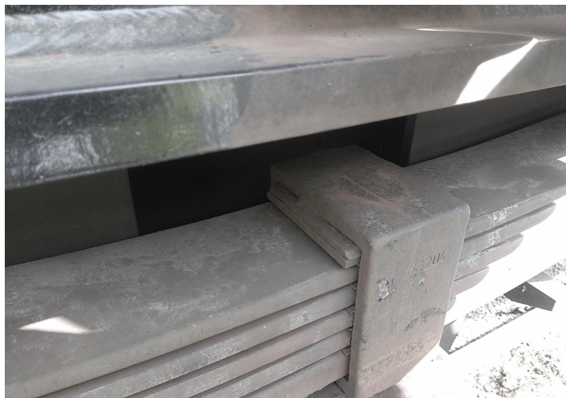
Figure 1. Two-axle wagon suspension with a parabolic leaf spring.
