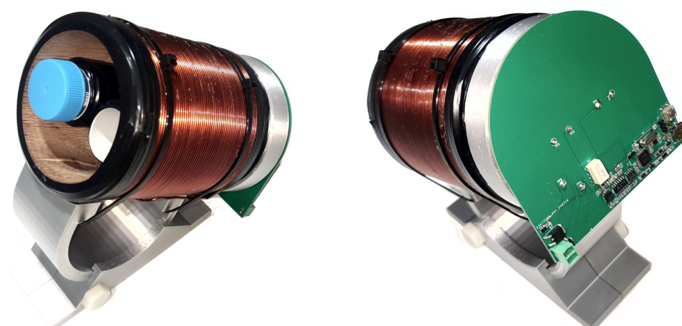
Figure 19. The final device was successfully assembled, integrating all components into a cohesive and fully functional EFNMR spectrometer.
