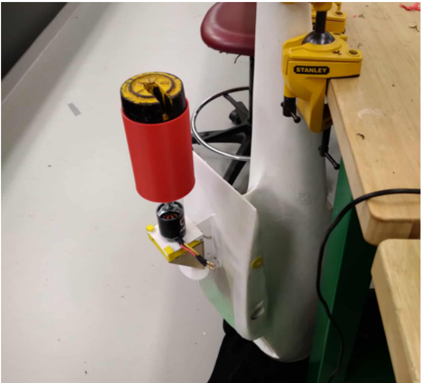
Figure A9. Thrust calibration setup (own photograph).
