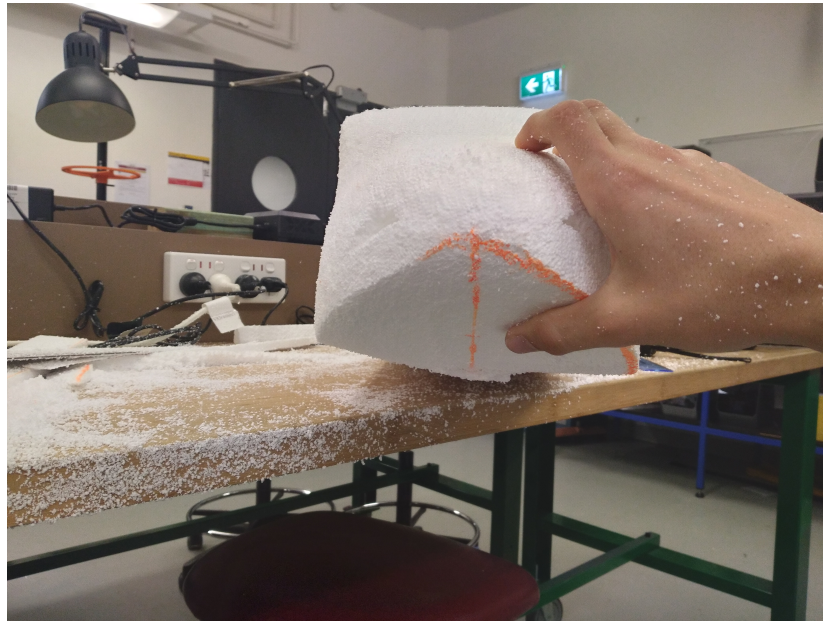
Figure A4. Fuselage front shaping in progress (own photograph).
