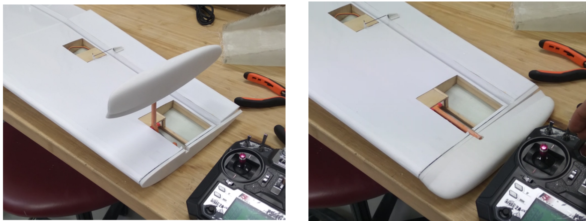
Figure 13. Extended and retracted wingtip pontoons (own photographs).
