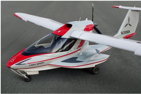
Figure 4. Icon A5 with fuselage-mounted pontoons (adapted from [8]).
