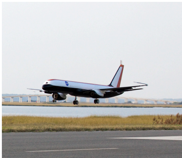
Figure 9. NASA AirSTAR 5.5%-scale loss of control research aircraft (adapted from [53]).
