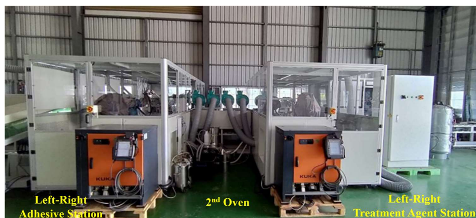
Figure 25. External view of the treatment agent and adhesive spraying station.
