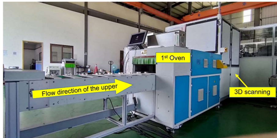
Figure 23. External view of the loading/drying and 3D scanning station.
