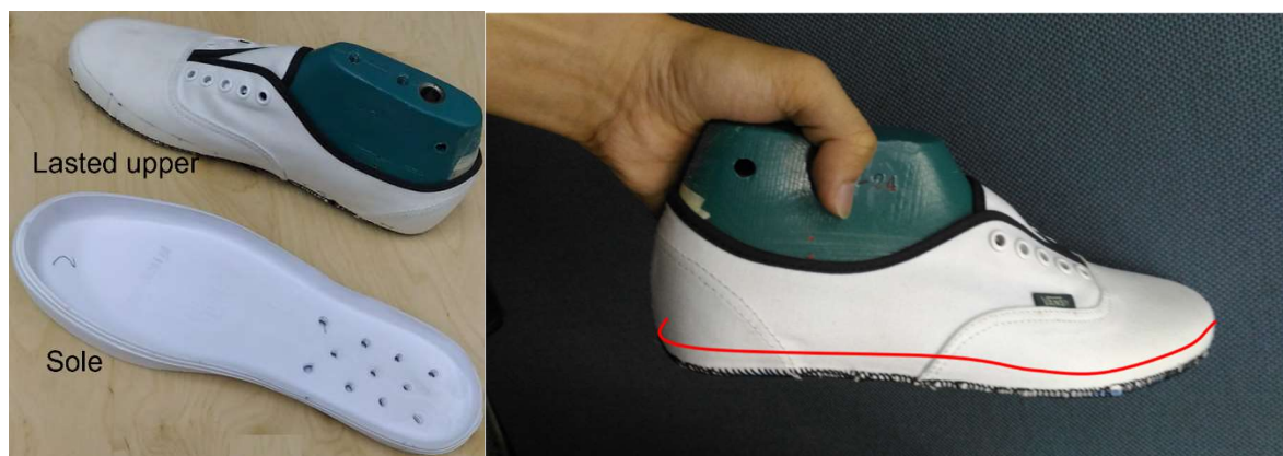
Figure 18. Schematic diagram showing the outsole and its corresponding bonding line on the lasted upper.
