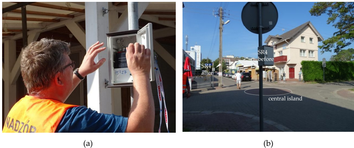
Figure 6. Survey station equipment (SR4): (a) traffic detection device; (b) SR4 sited before and after traffic circle. Source: photo by Alicja Sołowczuk.
