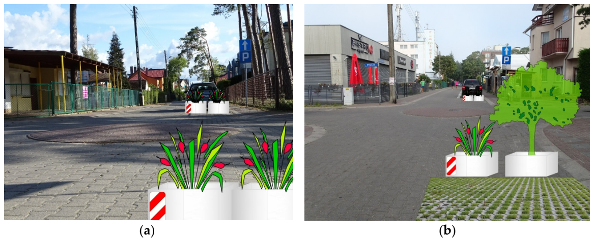
Figure A1. Visualization of the proposed traffic safety improvement measures using green infrastructure components suitable for home zone applications: (a) tree boxes with appropriately selected species used as side obstacles (greenery resistant to drought, frost, exhaust emissions); (b) side obstacles with appropriate grafted tree species. Source: elaboration own.
