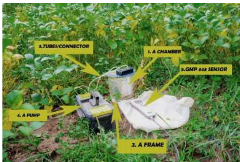
Figure 2. Field setup for soil respiration measurement using the closed chamber method.
