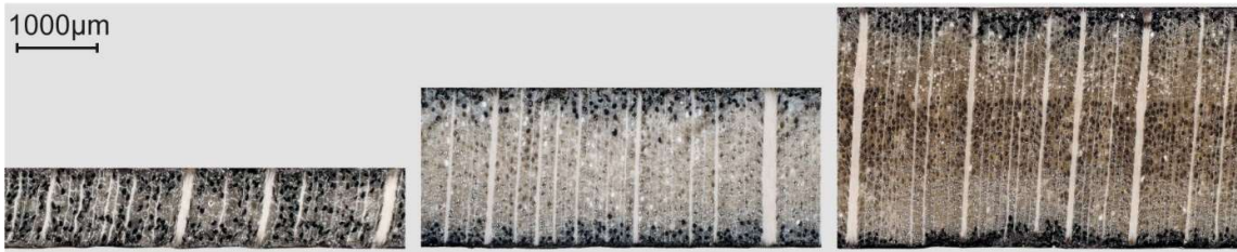
Figure 1. Qualitative comparison of the adhesive infiltration (black) in dependence on the veneer thickness: 1 mm (left); 2 mm (middle); 3 mm (right).
