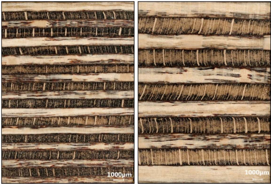
Figure 3. Microscopy of the plywood cross-section of 1mm (left) and 2mm veneer layers (right).
