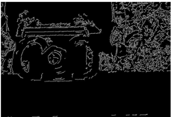
(c2) Improved Canny result for rusty surface
