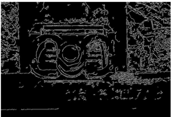
(b2) Improved Canny result for surface with water stains
