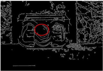
(b1) Traditional Canny result for surface with water stains
