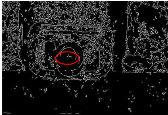
(d1) Traditional Canny result for surface with oil stains
