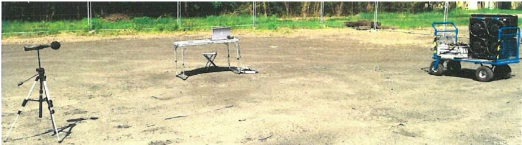
Figure 12. The view of the test stand during the performance of acoustic pressure tests of the radiator.
