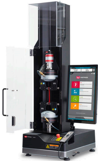
Figure 37. The Model 5965 UTM are designed to perform tensile, compression etc (www.instron.com).
