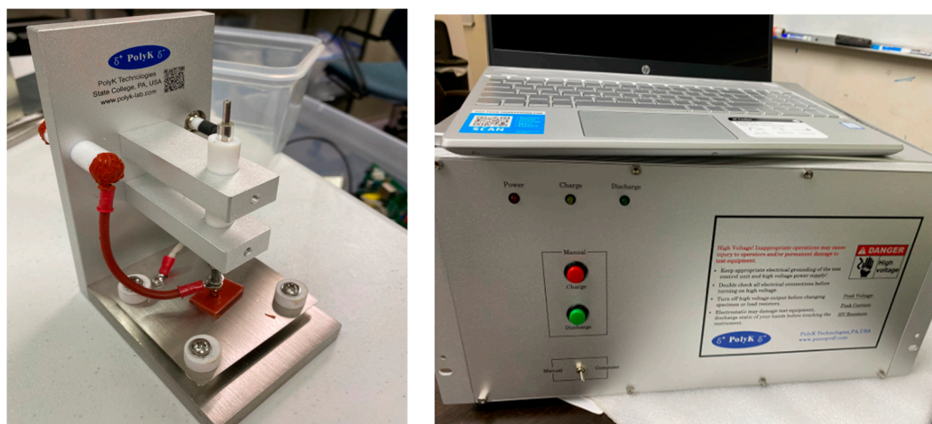
Figure 42. Dielectric test system a test fixture along with dielectric material charge system[55].
