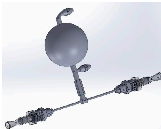
Figure 9. 3D Schematic of the Hydrazine Thruster Dual Cluster Feeding System.
