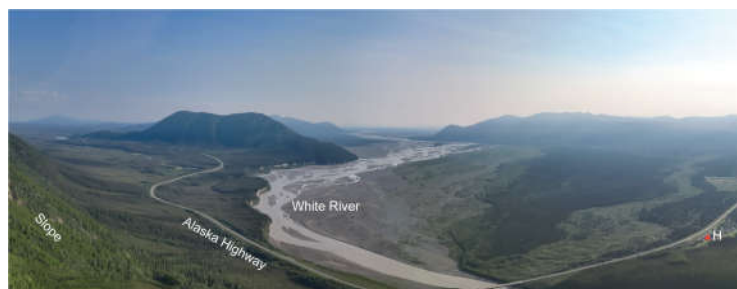
Figure 4. Panorama of two photographs taken at ~1060 m HAE by the M3TD. This shows how the aircraft must stay relatively close to the terrain (e.g., the slope seen on the left), while the home point (takeoff location) designated by the letter H is 350 m below (lower right).
