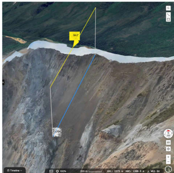
Figure 7. Screen capture from FlightHub 2 displaying the July 14 th model illustrating the slope estimated to be 34.2°.
