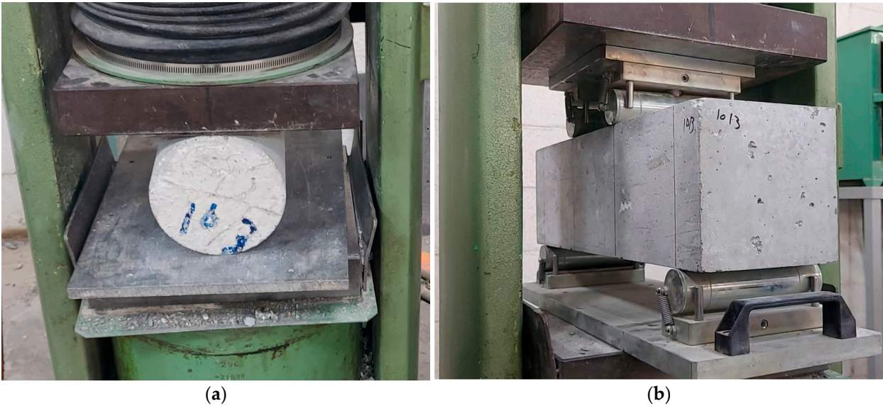
Figure 2. (a) Concrete splitting tensile strength test. (b) Concrete Prism test.
