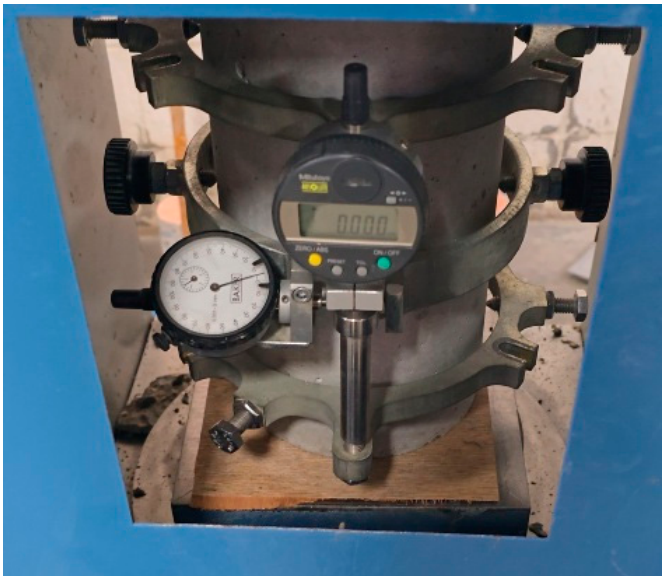
Figure 3. Concrete static modulus of elasticity test.
