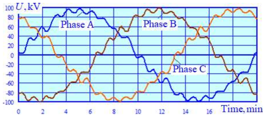
Figure 21. Voltage curve shapes on 110 kV buses of TS 3 at the 37 th minute of modeling.
