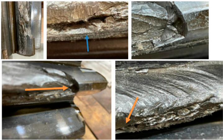
Figure 18. Sun shaft – arrows show material separation.
