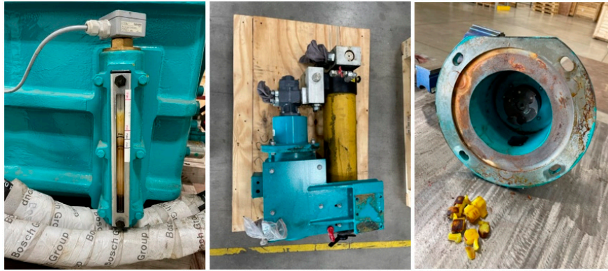
Figure 10. Lubrication system ( left ) foam into the oil ( mid ), coupling spider slattered ( right ).
