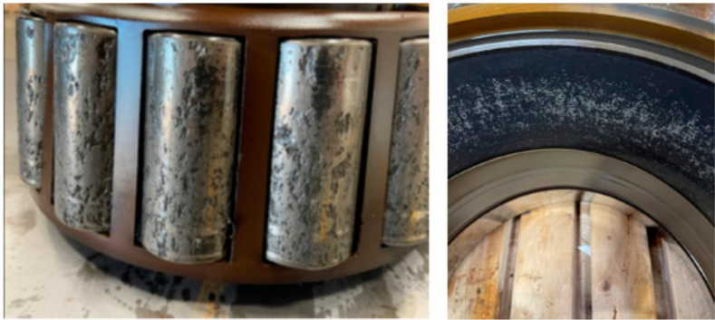
Figure 16. View of the planet gear bearing.
