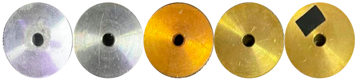
Figure 1. From left to right: aluminum, steel, copper, bronze, and brass (marked with black duct tape for better distinction due to its similarity to bronze) cylinders, viewed from above.
