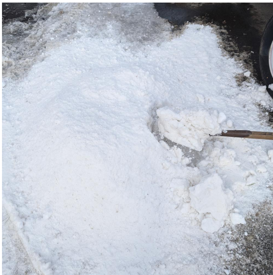
Figure 2. Naturally occurring source snow after being processed with a snowblower prior to being added to the CEB machine hopper.
