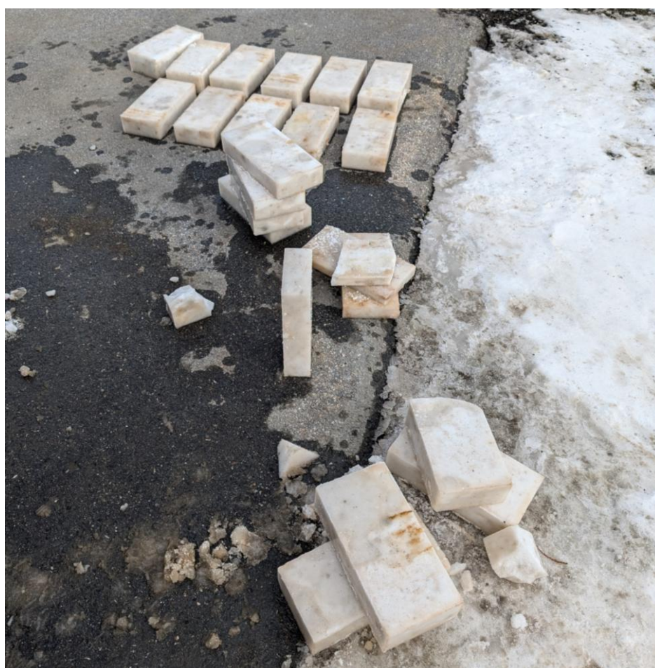
Figure 3. A mixture of successful (background) and unsuccessful (mid- and foreground) compressed snow blocks (CSBs) produced by the Impact 2001A machine. Unsuccessful blocks are those that failed upon being ejected from the machine or were not produced at the correct block height. Successful blocks are those within 1 cm of the intended block height setting.
