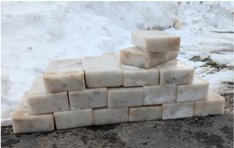
Figure 4. Successful, but not uniform, CSBs produced by the Impact 2001A machine. Some of these blocks were produced during the first 3-4 cycles after block height adjustment, so the actual block height is more than 1 cm larger or smaller than intended.
